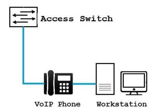
You have configured 802.1X single supplicant mode on the access switch. The VoIP phone does not support 802.1X authentication.
