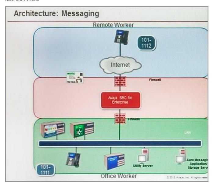
Avaya Tier 3 support receives a case escalated by Tier 2 where the customer cannot receive incoming calls, but can make calls out successfully. The trace shows that the incoming calls arrive at the Avaya Session Border Controller for Enterprise (SBCE) but fail to get routed into the customer enterprise network.
