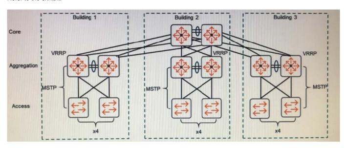
A customer wants to replace the core and aggregation layer of an existing network. Currently the network routes between the aggregation layer and core, and uses the technologies shown in the exhibit.
