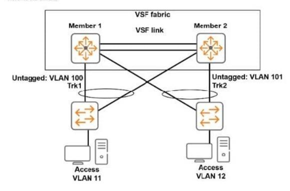
The Virtual Switching Framework (VSF) fabric and other switches connect on LACP link aggregations. They use OSPF for routing. What should a network administrator do to help network connectivity continue uninterrupted if the commander fails?
