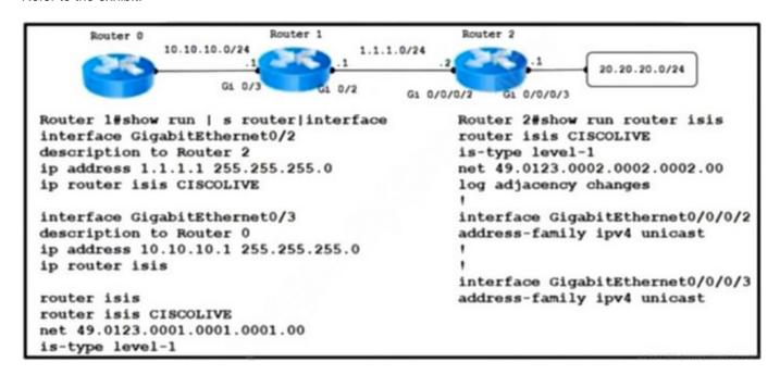
An engineer is troubleshooting a network routing issue on this IS-IS network situated at the customer\\'s regional hub. Router 2 that runs Cisco IOS XR Software cannot see the network 10.10.10.0/24 on router 1. The Layer 2 encapsulations are correct. The ARP connectivity for the Ethernet interface that runs IS-IS is working. Which action resolves the issue?
