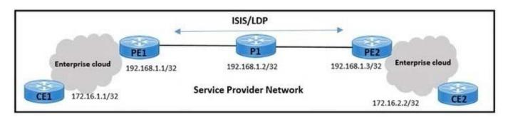
An engineer working for a private telecommunication company with an employee id 4115 46 881 is enabling a segment routing solution with these requirements. A service provider is using the default range for prefix SID. PE1 must allocate the first SID from the default range for the loopback address PE1 and PE2 loopback SID allocation should have a minimum difference of 500.
