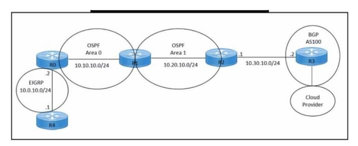
An engineer must redistribute only the 10.0.10.0/24 network into BGP to connect an on-premises network to a public cloud provider. These routes are currently redistributed:
